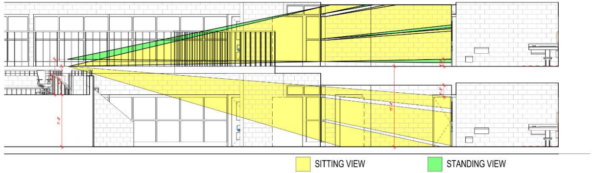
1 BUILDING SECTION @ OPTION 2 - VISIBILITY OF CELLS FROM CONTROL STATION - FLOOR RAISED 7'-4" SCALE: 1/4" = 1'-0"
